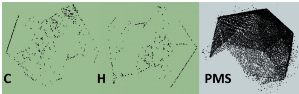
Fig 7. A cloud of points for the model created with the SUSAN operator from two photographs taken with the Canon 20D - (C) and Hasselblad H4D50 - (H). For comparison a model created by the PhotoModeler Scanner - (PMS) is presented.
